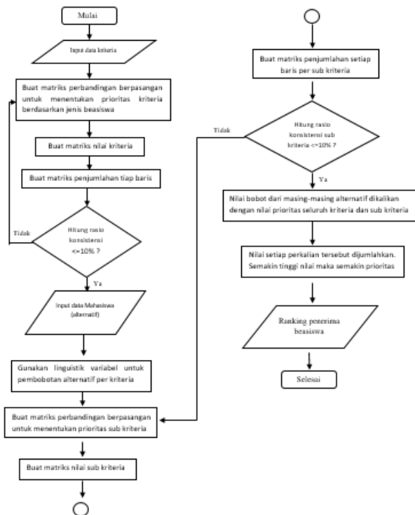
Gambar 2.65 Flowchart Proses AHP
